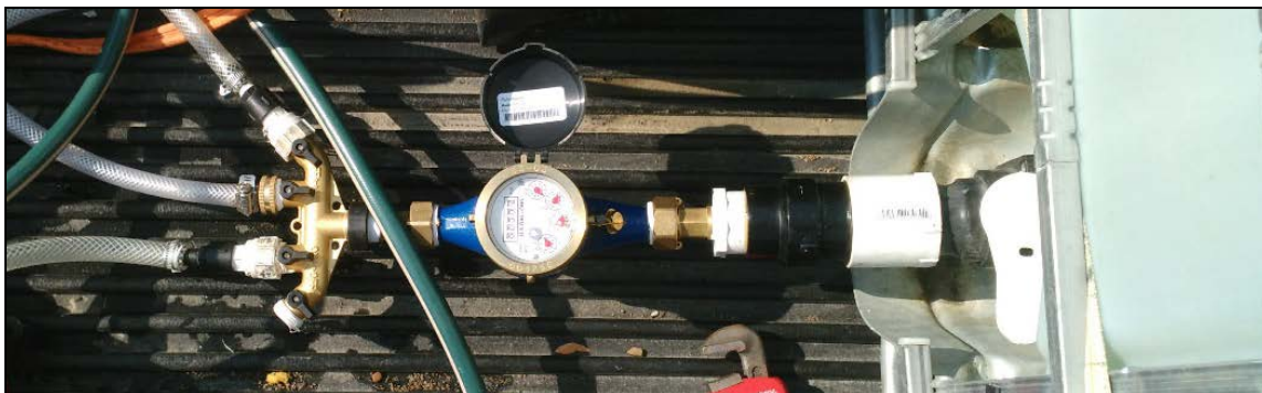
FIGURE 28 Photograph of the new inline water meter used to log water flow during VEI scanning.
