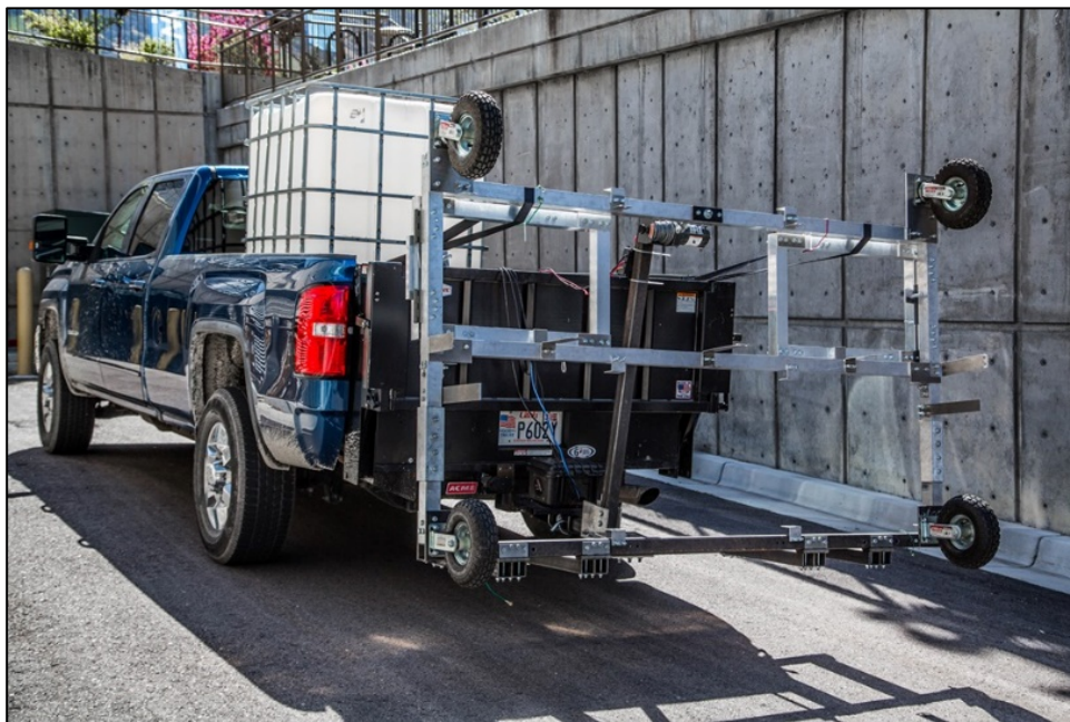
FIGURE 6 Photograph of VEI scanner reduced in overall size and folded up for transport over long distances.
