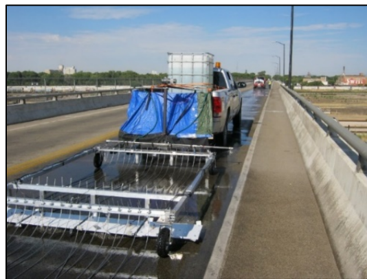
FIGURE 23 Photograph of VEI scanner deployed on the longest bridge deck in Utah.
