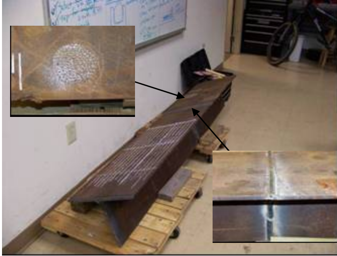
FIGURE 10 Spliced pile with wall loss located beyond the defect
