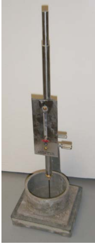
FIGURE 4 Vicat apparatus for mortar set time testing.
