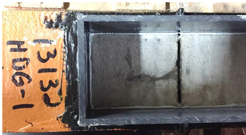
FIGURE 15 Crack on one of four HDG minibeam that cracked in testing.
