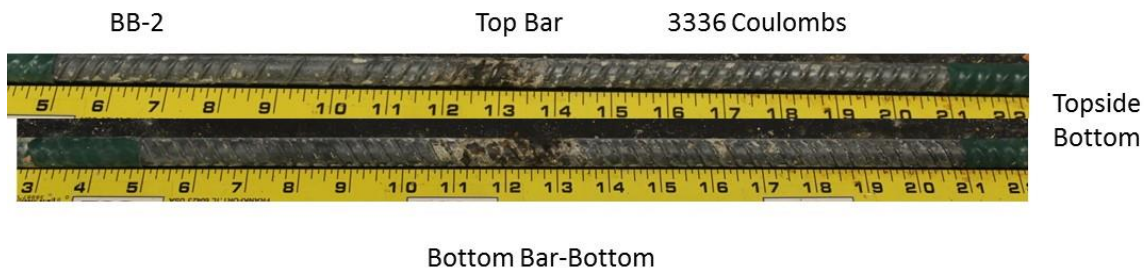
FIGURE 16 BB-2 bars after 34 cycles (68 weeks) of corrosion testing.
