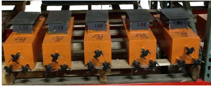
FIGURE 6 Cracked beam corrosion specimens. Specimens are 6 in. x 6 in x 20 in.
