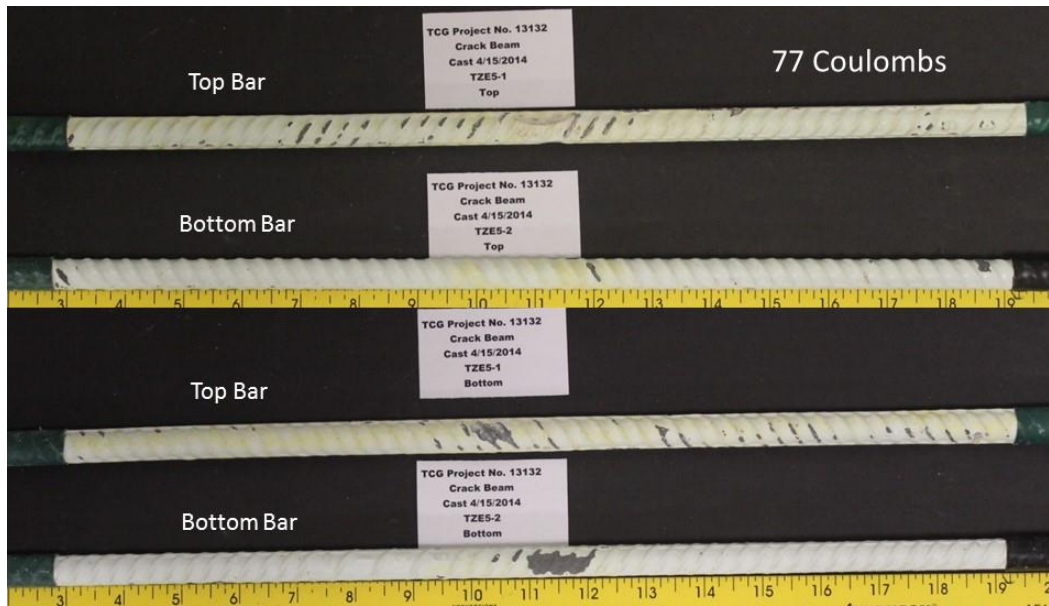
FIGURE 22 TZE-4 bars after 36 cycles (72 weeks) of corrosion testing.
