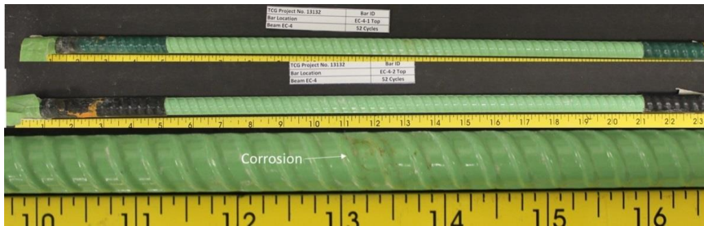
FIGURE 27 ECR-4 bars after 52 cycles. Bar 1 on top and magnified or the top bar, bar 2 is a bottom mat bar.
