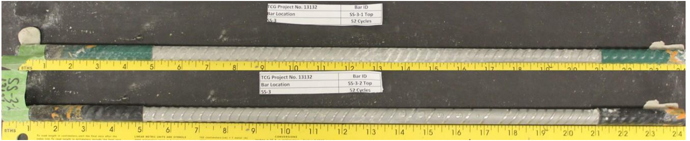
FIGURE 29 SS-3 bars after 52 cycles. Bar 1 is the top bar and bar 2 is a bottom mat bar.
