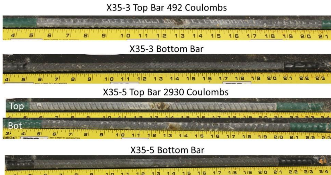
FIGURE 19 X35 bars after 34 cycles (68 weeks) of corrosion testing.
