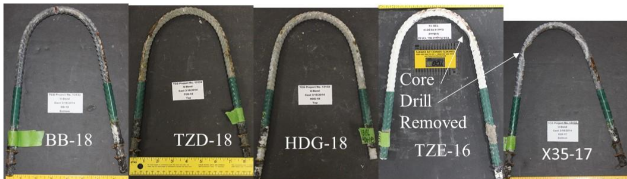
FIGURE 42 Typical corroding bars at the end of testing.
