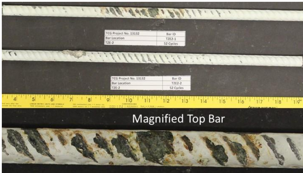
FIGURE 26 TZE-2 bars after 52 cycles. Bar 1 is the top bar and bar 2 is a bottom mat bar.
