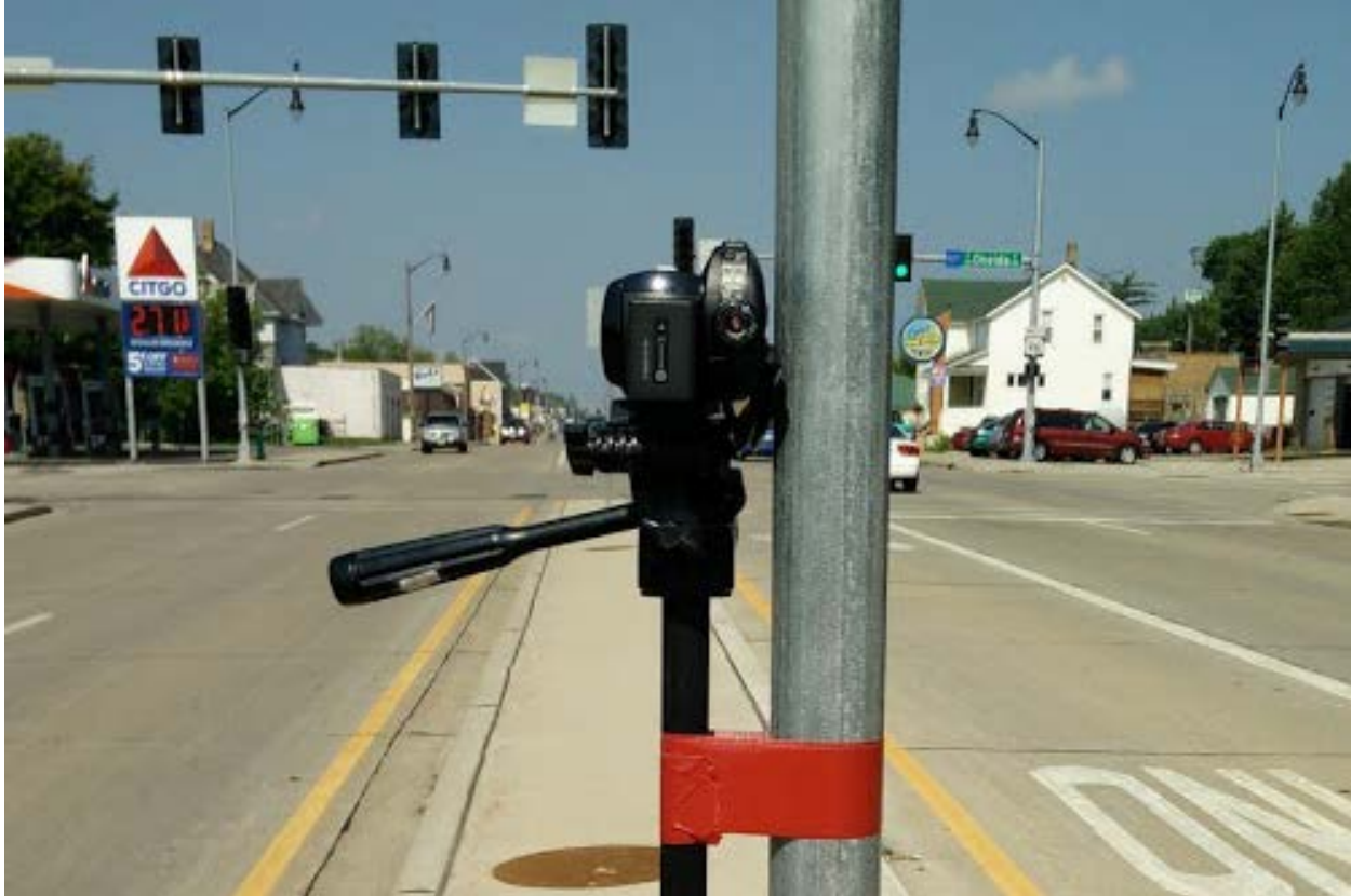
Figure 10. Camera mount used for video recording at supplemental data collection sites.
