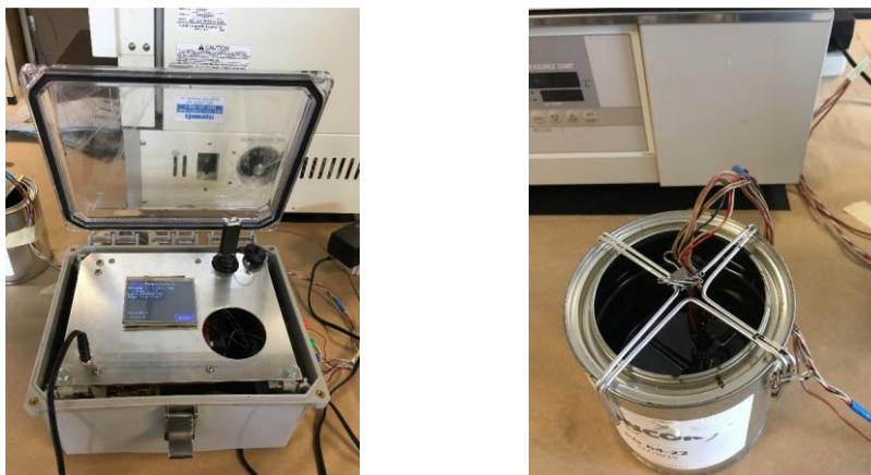
Figure 17. DART prototype for field testing and binder testing setup.
