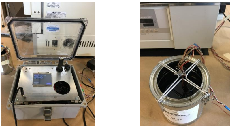
Figure 1. DART prototype for field testing and binder testing setup.
