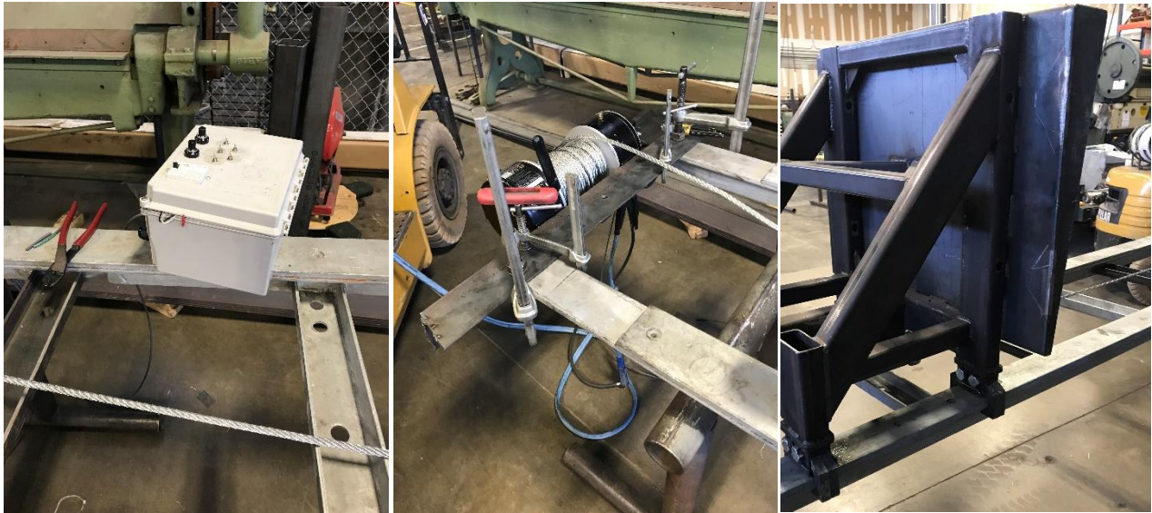
FIGURE 9 Bench testing set up: (left) PLC; (middle) winch; (right) sled and feet
