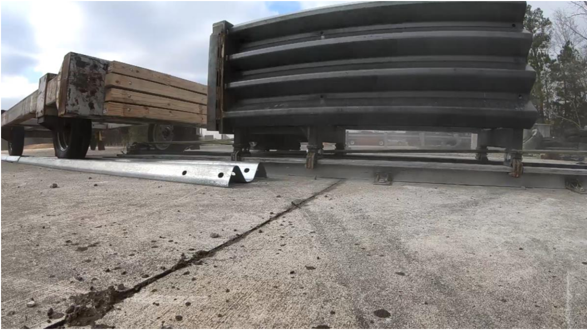
Figure F 3 - Position after spring back for test 4
