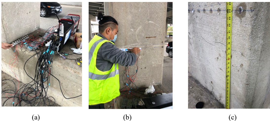
FIGURE 24 The challenges faced at the field measurement: (a) cabling; (b) coupling; and (c) ensuring direct path between transmitters and receivers.
