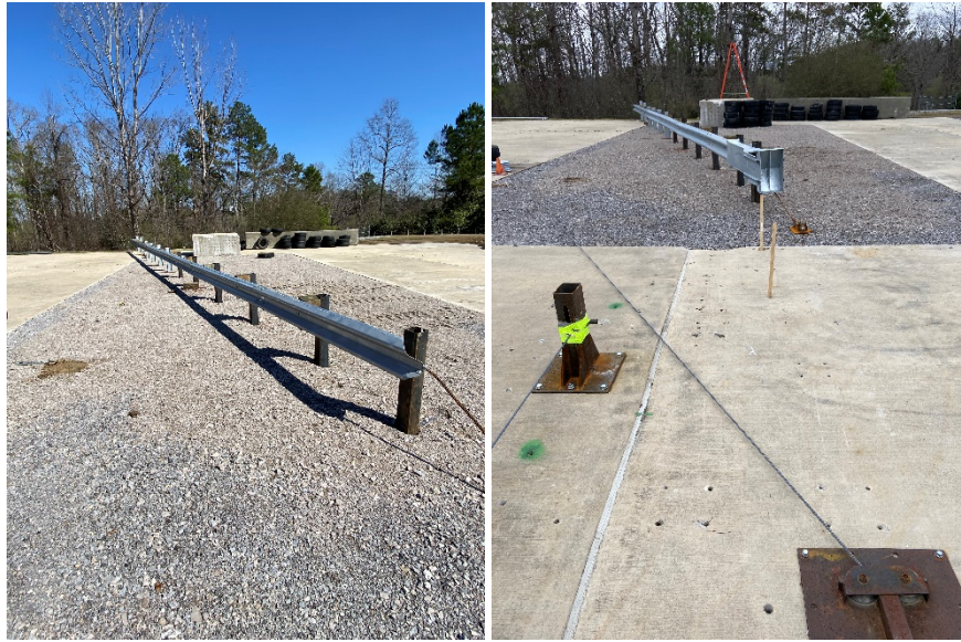
FIGURE 14 Test setup (left) without terminal head and (right) with terminal head
