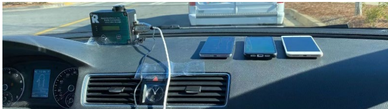
Figure 11. Picture. Device setup for multi-device sensor repeatability test.
