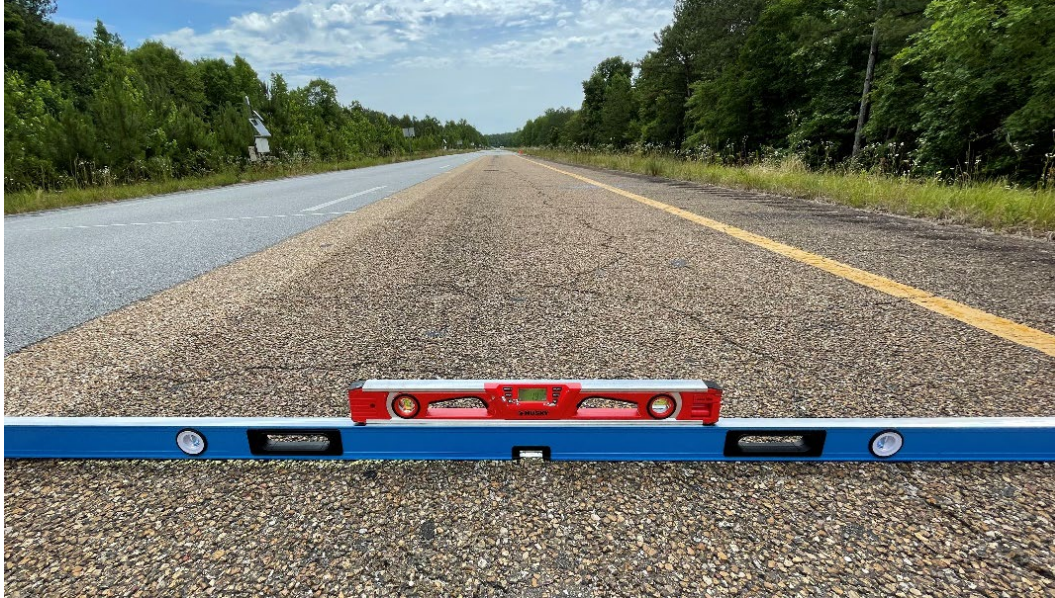
Figure 14. Picture. Straightedge and digital level used for superelevation measurements.
