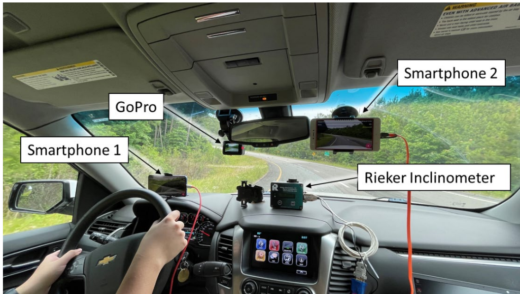
Figure 15. Picture. Mobile devices used in the validation test and their setup.
