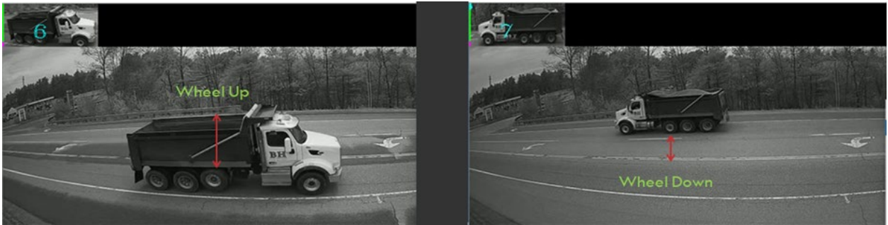
FIGURE 10 Wheel Up and Down Will Classify Differently
