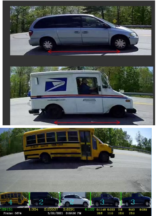
FIGURE 9 Wheel Based Classification Will Misclassify
