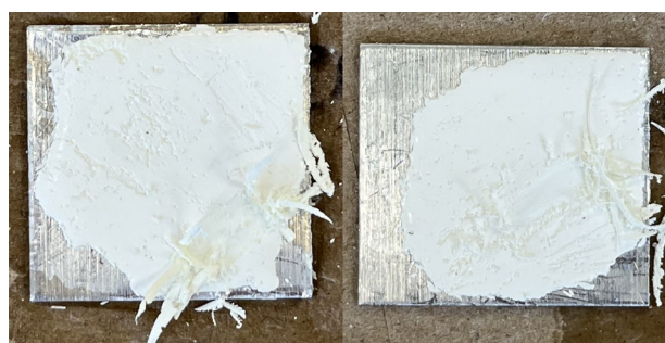
FIGURE 32. Surface roughness of 3-40/5-40/D-20 (left) and 4-55/5-25/D-20 (right) after being submerged in 5% acetic acid for 45 minutes.
