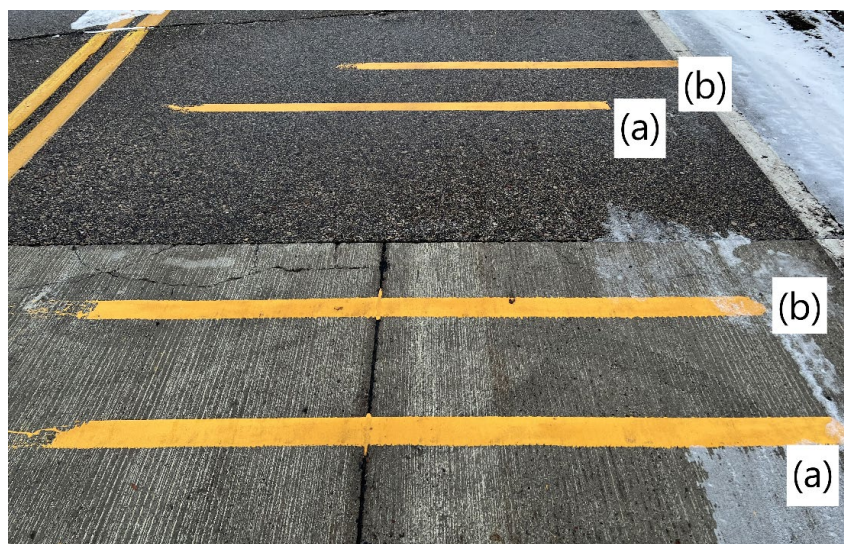
FIGURE 45. Markings of (a) 4-55/5-25/D-20 and (b) commercial formulations on the MnROAD test track after 6 months of low-volume traffic.
