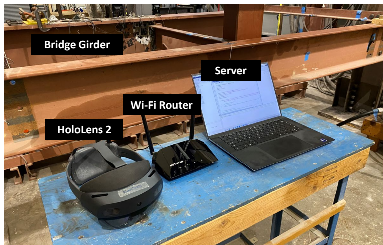
Figure 58 Hardware used in AR-based fatigue crack inspection
