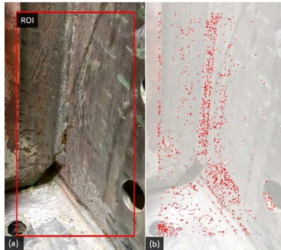
Figure 17 The initial frame of the 3D video with ROI (a): and all feature points detected by the Shi-Tomasi algorithm (b). Note that the brightness of image in (b) is enhanced to highlight the feature points
