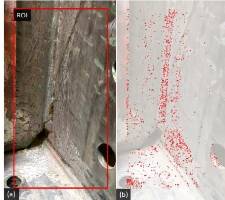
Figure 33: The initial frame of the 3D video with ROI (a) and all feature points detected by the Shi-Tomasi algorithm (b). Note that the brightness of image in (b) is enhanced to highlight the feature points
