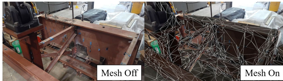
Figure 46 Visual mesh button reveals the HL2’s representation of real-world surfaces steel girder test
