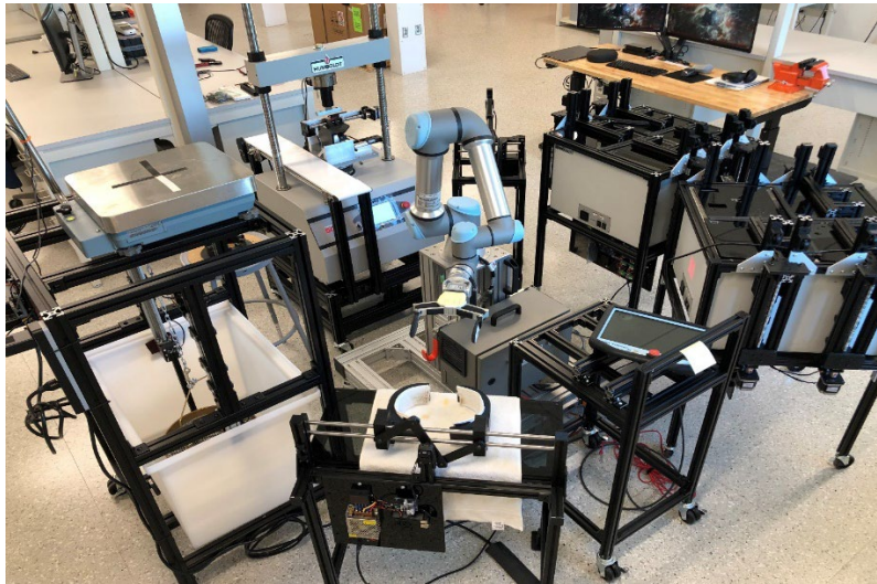
FIGURE 1 Asphalt mixture automated testing system with zero intervention (AMAZE).
