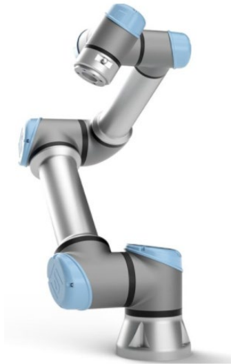
FIGURE 24 Robot arm: UR5e.
