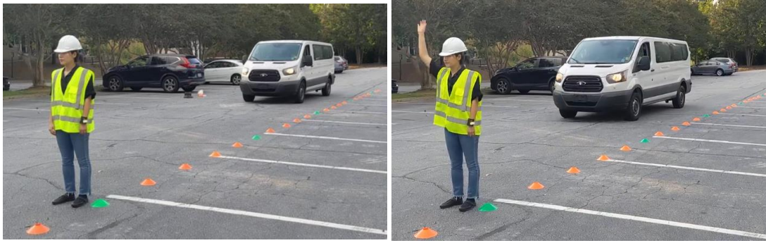
FIGURE 15 The mobile vehicle approaches the static worker from behind, and the worker raises their hand, indicating they sensed an alert from the PPU
