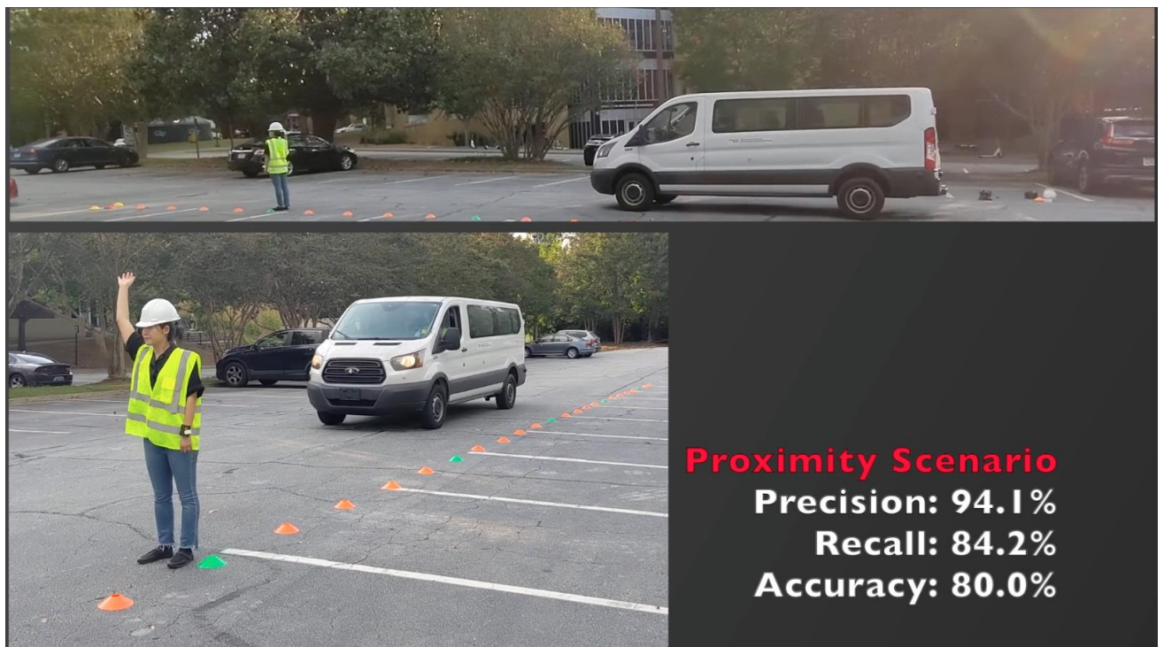
FIGURE Outdoor trials of the smart proximity alert system; evaluation of alerting functionality for hazardous situations
