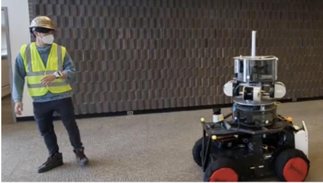
FIGURE 11 A worker with PPU and an EPU-attached mobile robot for proximity safety alerting test (i.e., During COVID)
