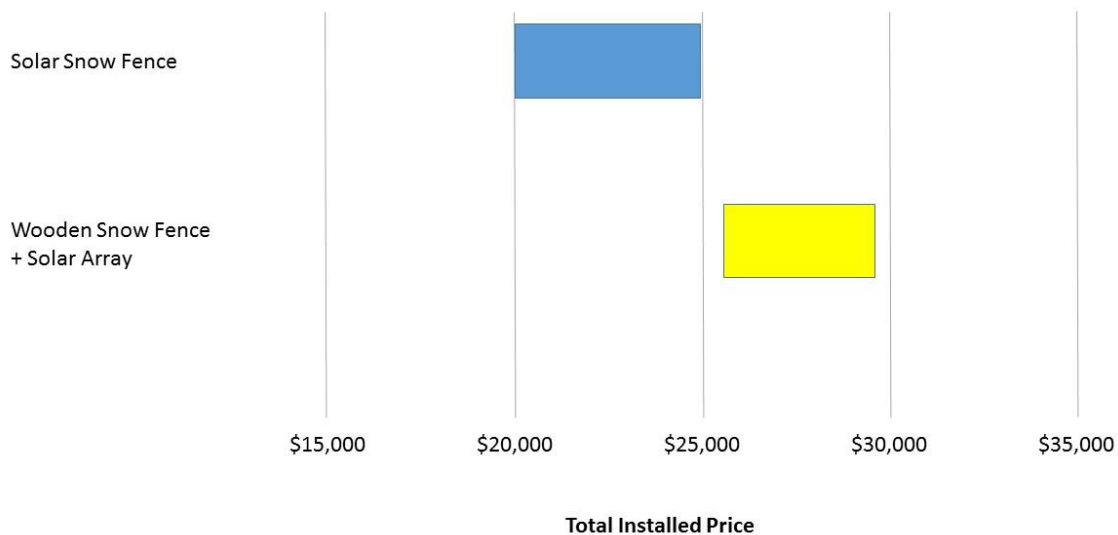
FIGURE 30: Range of CAPEX comparison of a dual use structure (solar snow fence – blue bar), a wooden snow fence and associated roof mounted solar array (yellow bar).
