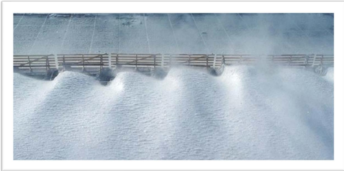
FIGURE 22: Effect of a 6 inch gap between snow fence panels on downwind snowdrift formation; resulting in reduced fence efficiency. (Image from (12)).
