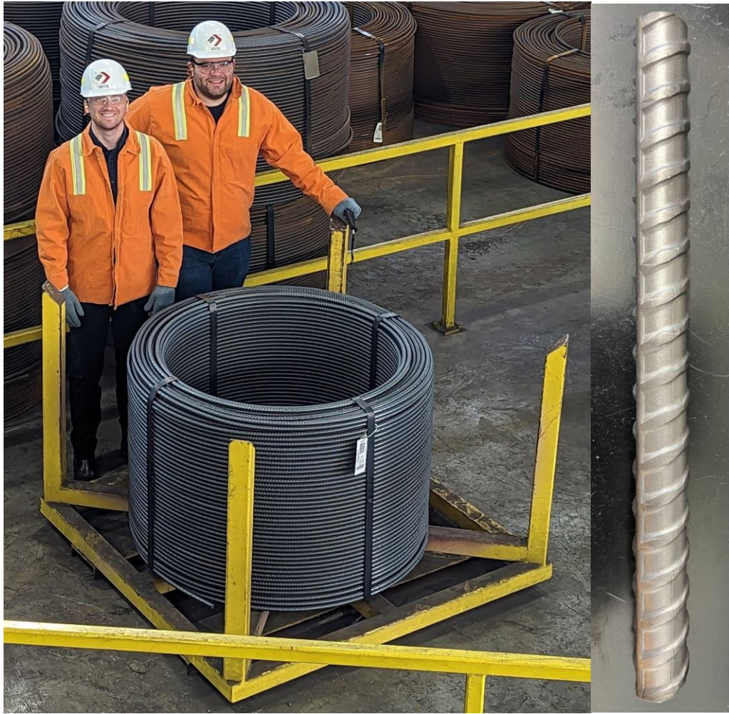
FIGURE 14: (Left) Allium co-founders with first large-scale batch (Right) Produced bar after abrasive blast cleaning
