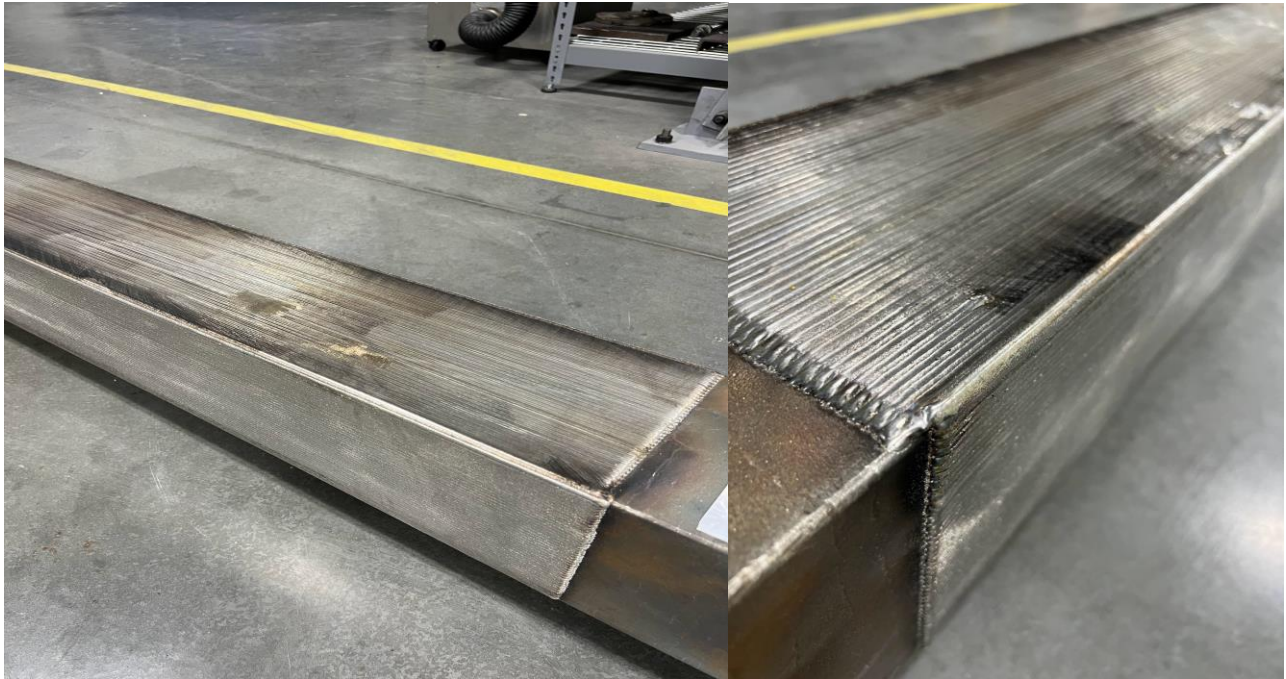
Figure 13: Pictures of the laser cladded billet, note that only the middle 10 feet of the 26 foot long billet were cladded. The cladding is approximately \frac{1}{8} " thick.
