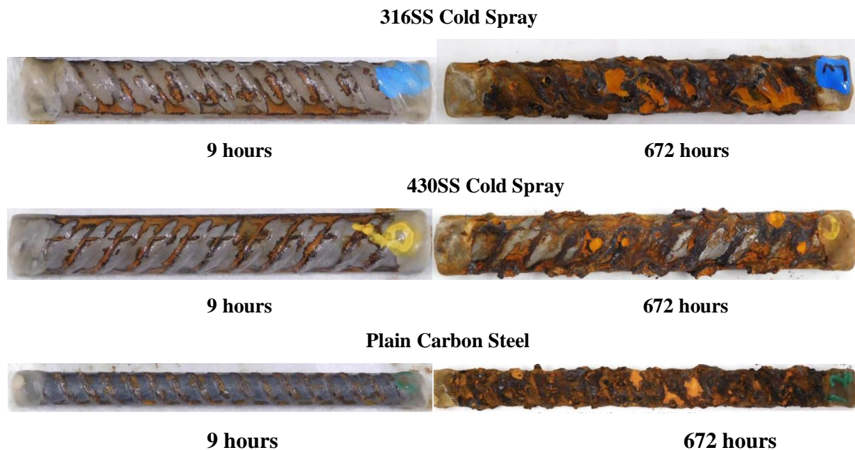
FIGURE 3 Photographs of cold spray coated rebar samples after 9 hours (left) and 672 hours (right) of salt spray testing (ASTM B117). Note the corrosion attack emanating out from the top and bottom ridges of the coated rebar.
