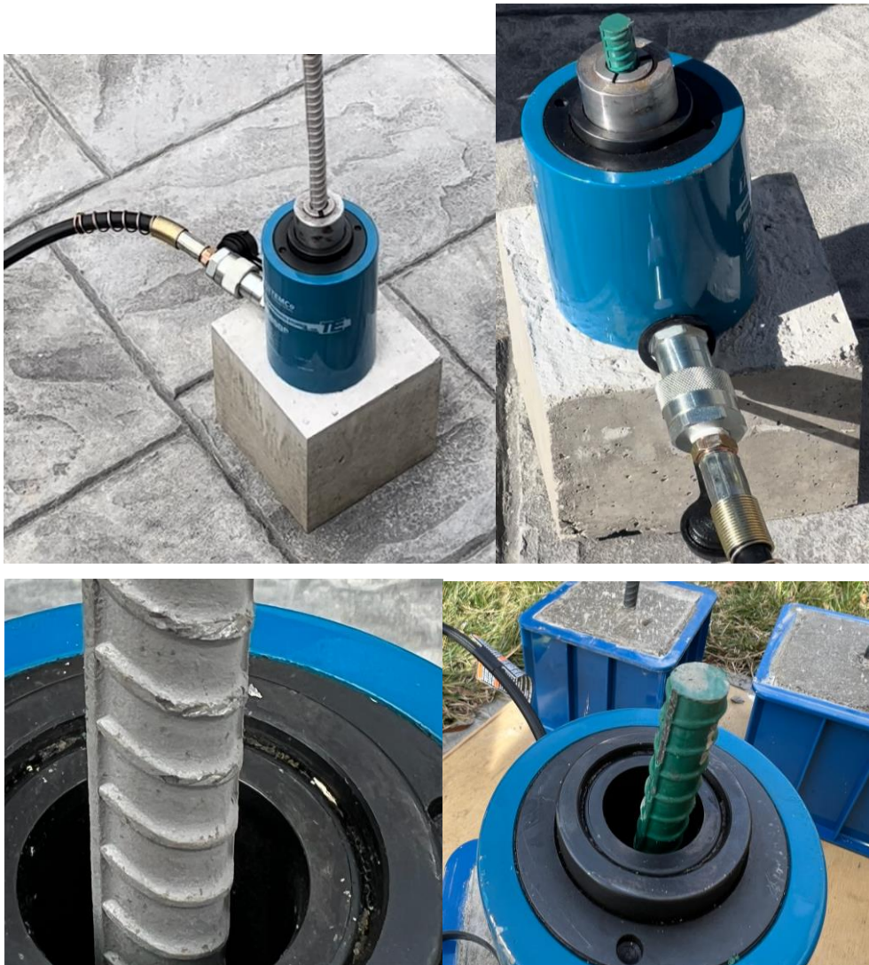
FIGURE 22 (Top Left) Pullout test of rebar coated with stainless steel using cold spray coating (Top Right) Pullout test of epoxy-coated rebar (Bottom Left) Threading marks left on cold spray coating after pullout testing (Bottom Right) Epoxy-coating removal and damage due to threaded wedges used during pullout testing.
