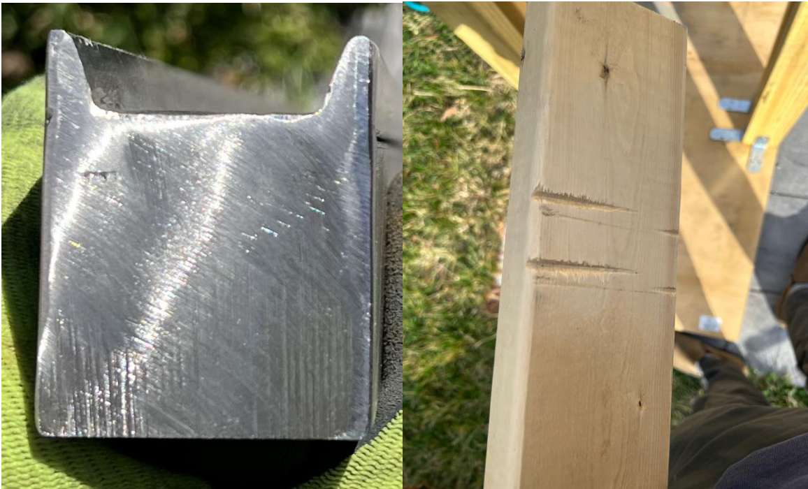
Figure 24: (Left) Custom weighted channel bar used for creating damage (Right) example of damage level caused by drop onto 2x4 piece of wood.
