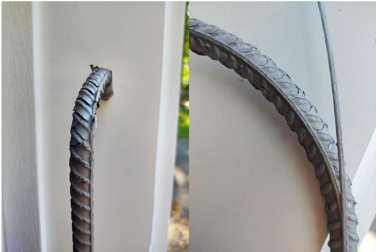
FIGURE 8 430-coated rebar after 90 degree bend test showing periodic cracking along the diagonal ribs (left) and along the long ridge of the rebar (right). The results indicate minimal coating ductility in the as-sprayed state.
