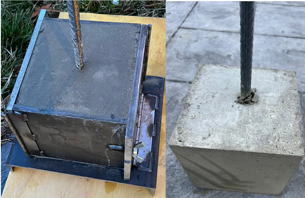
FIGURE 23 (Left) Black rebar specimen being cast in 6-inch cube reusable steel mold. (Right) Characteristic damage after pullout failure.
