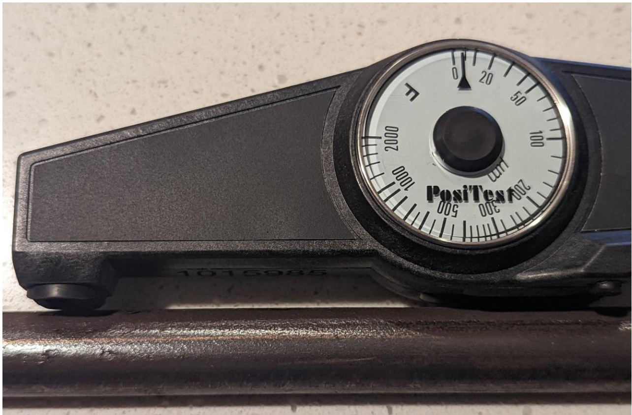
FIGURE 26 A hand-held magnetic gauge which can measure average coating thickness within a ~1mm diameter measurement spot, and can also identify cladding/coating breaches in non-magnetic stainless steel coatings.
