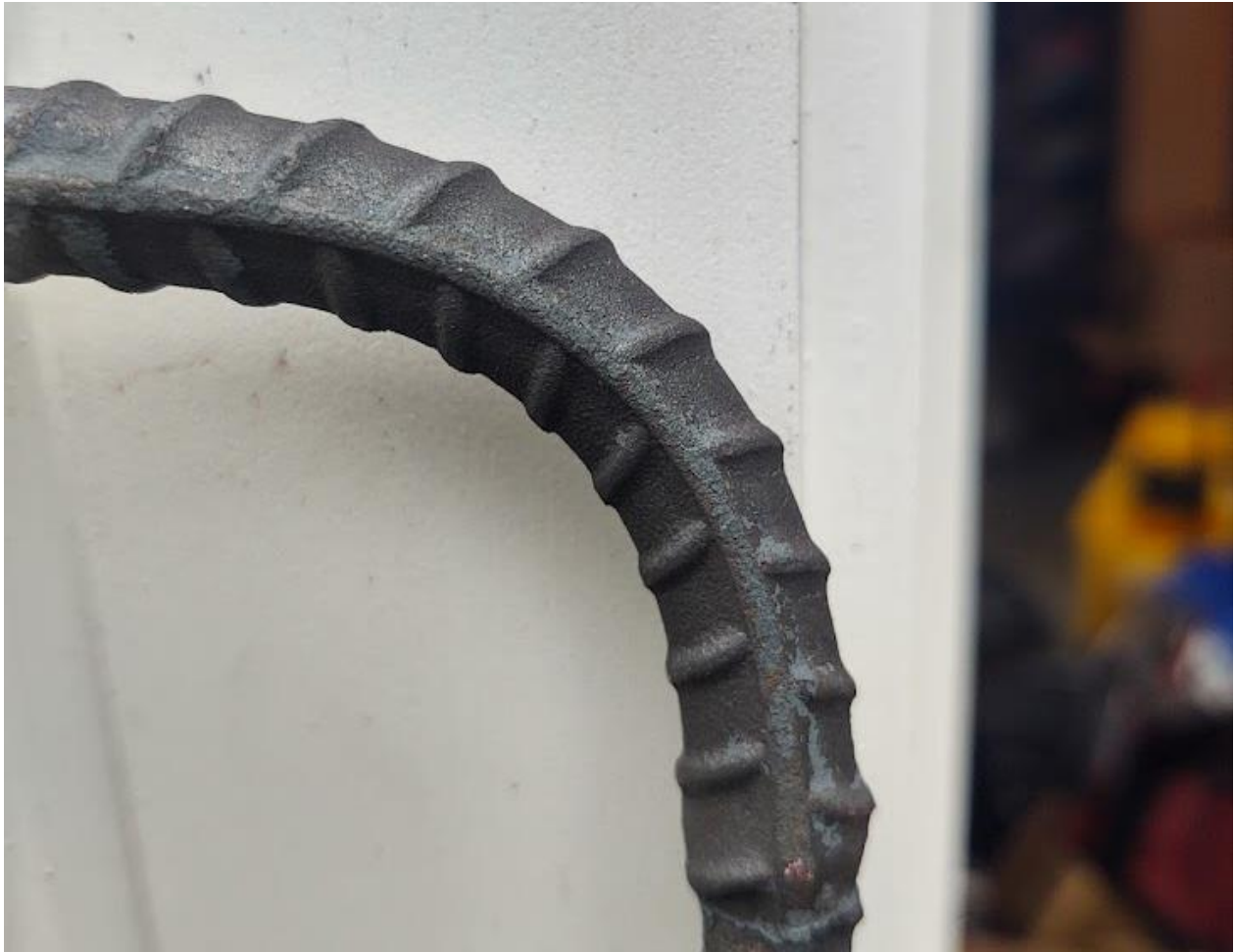
FIGURE 9 S220 coated and thermally treated rebar after 90 degree bend testing. Note that the slight dark discoloration is due to high temperature oxidation during the thermal treatment. The bar is able to bend without any perceivable cracking in the coating.
