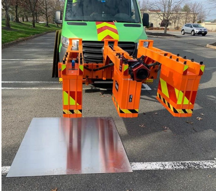
Figure 4-Metal plate calibration in the field
