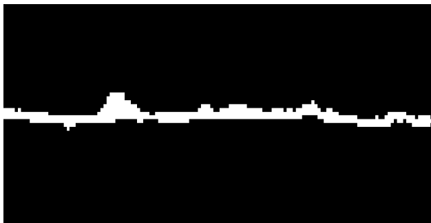
Figure 4-6 Crack block image from 5x5 block processing.
