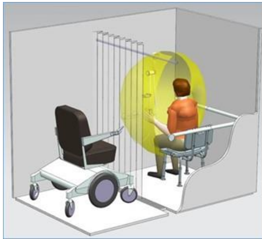
Figure 6 Reach study with 5 th percentile female manikin using a shower chair in bi-level shower.
