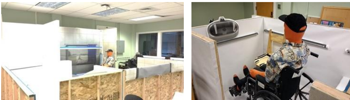
Figure 1 Images of the constructed full-scale soft mock-up shown with a 50 th percentile male manikin in a manual wheelchair.
