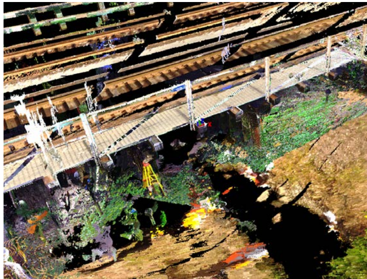
FIGURE 11. 3D Laser Scan of SV 849.9 Bridge
