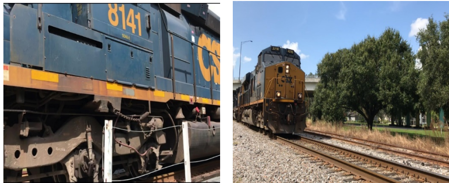
FIGURE 8. CSX 6 Axle-Locomotive (Freight Train) used for dynamic load testing in SV 849.9
