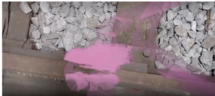
Figure 22. Vision coverage results of rail track inspection (ARRA-Eye software interface).
