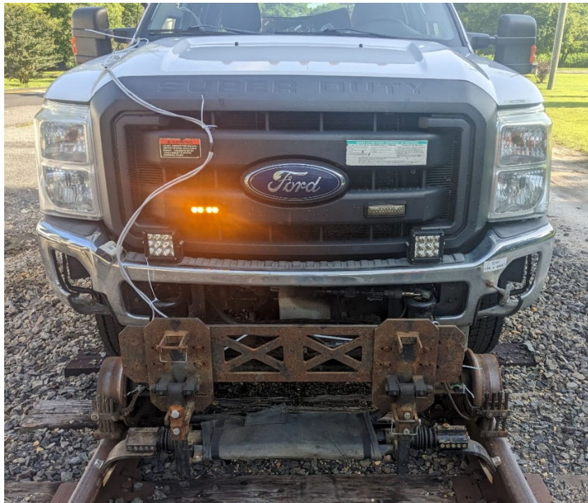
a) Front of vehicle showing cabling and contact gage measuring system
