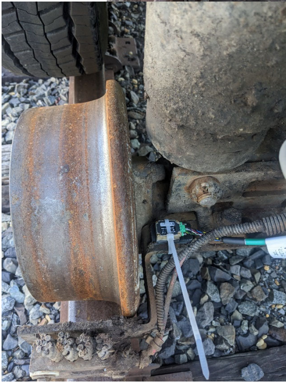
SmartWheel sensor installed on left and right guide wheels of hy-rail vehicle
