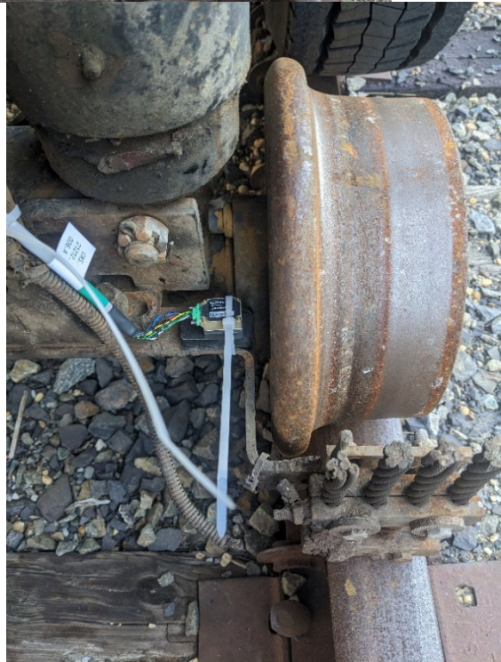
SmartWheel sensor installed on left and right guide wheels of hy-rail vehicle
