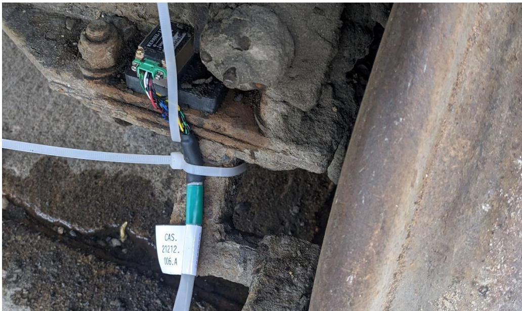
b) Sensor tethering to rear of cab
