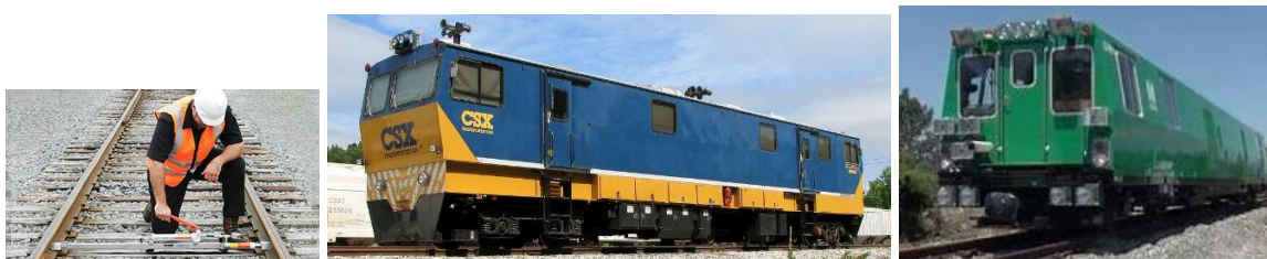
Figure 7: Dynamic tools used today, PTLF, GRMS and Geometry Car
