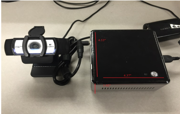
Figure 2: Depiction of our portable driving monitoring system parts.
