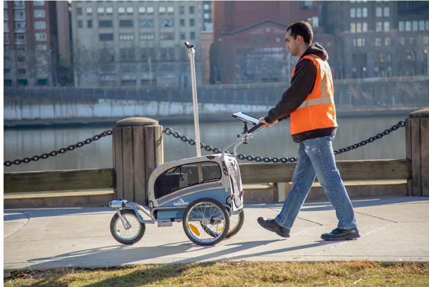
Figure 1: PathMeT is a portable microcontroller-based system that includes an accelerometer, inclinometer, laser, camera and GPS.
