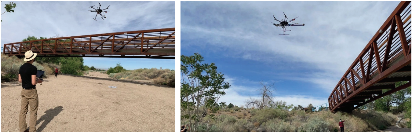
Figure 2. First real bridge test with untethered wireless outdoor UAV-Laser-Camera testing for measuring contact-free, reference-free displacements (Albuquerque, New Mexico): (a) pilot control and (b) drone laser solution lateral view.
