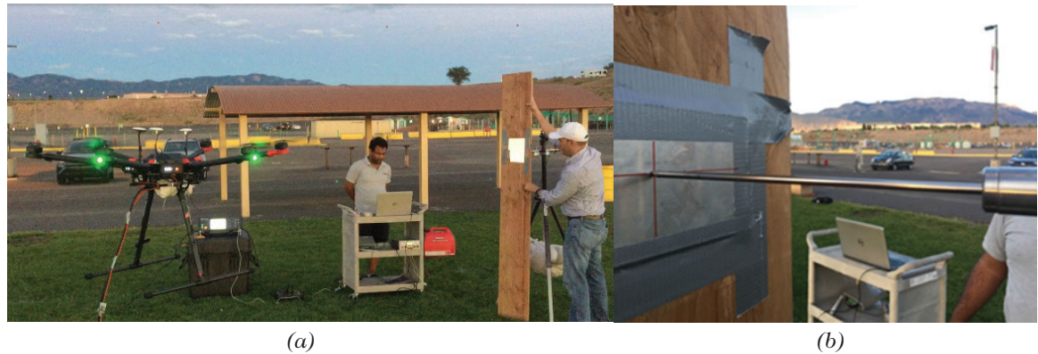
Figure 1: First outdoor laser UAV testing for measuring contact-free, reference-free displacements compared with reference displacements: (a) experiment general view; (b) reference displacement detailed view.
