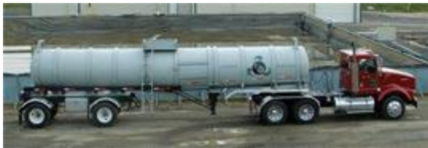
Figure 2. Tanker for transport of high-concentrate glycol to an off-site recycling facility.
