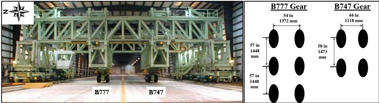
Figure 2. NAPTF Test Machine and Landing Gear (photo courtesy of FAA NAPTF)
