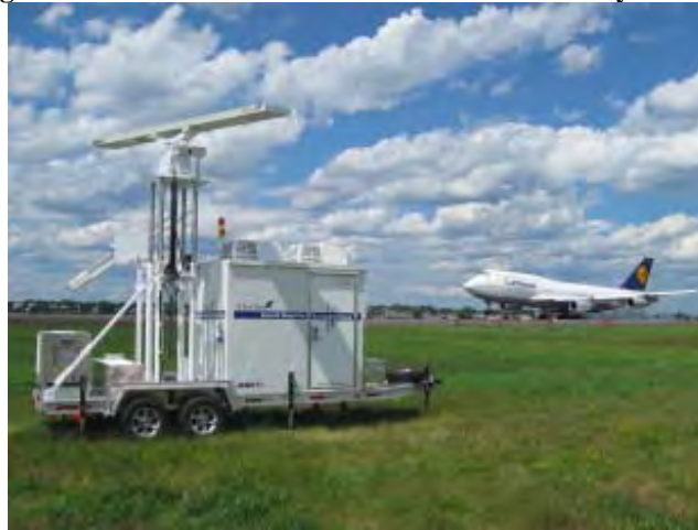
Figure 4: MERLIN Bird Strike Avoidance Radar System
