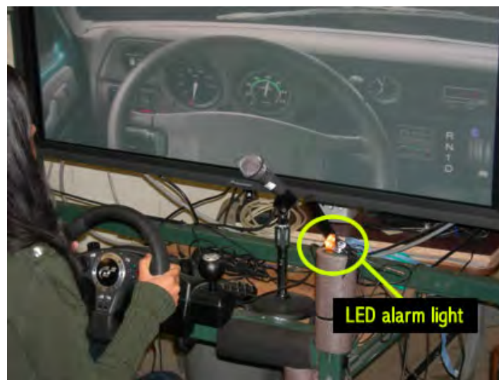
Figure 3-2. Picture of the visual alarm placement on simulator
