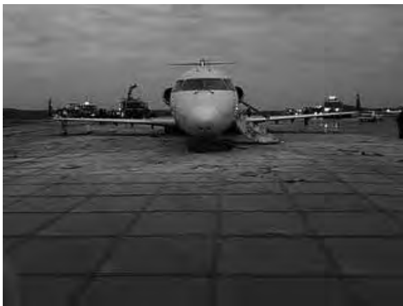
Figure 2 EMAS blocks collapsed to stop a plane that overshot a runway [9].
