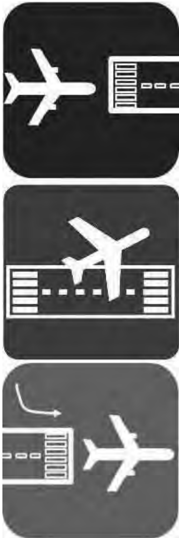
Figure 1 Runway excursion depictions from top to bottom: runway undershoot, runway veer-off and runway overrun. [5]
