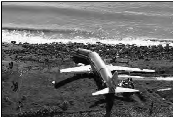
Figure 25 American Airlines flight 331 overran the runway at Norman Manley Airport and split in half.[62]
