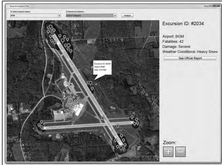
Figure 11. Proposed output of the Excursion Analysis Tool. The red dots display excursions that occurred at BGM. The orange dots are excursions that occurred at other airports of a given category, as if they had occurred at BGM. On the right is where data selected on the map is displayed. The red coloring indicates areas at high risk of
