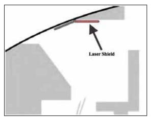
In the event of a laser attack, a pilot may reach overhead and lower the laser shield. This maneuver is an intuitive and natural reaction, as a pilot would lower a sun visor in a similar way in response to sun glare.
