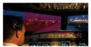
**Figure 15** - The location of the visor, shown in red, is designed to cover the area highlighted in Figure 14 [35]
