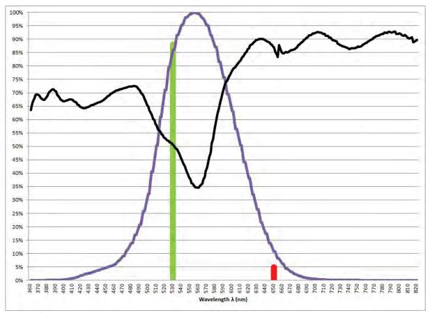
**Figure 12** - Frequency of laser attacks are shown in their respective wavelengths [33] (for red and green lasers). Relative human eye sensitivity is emphasized in purple [31]. The polyester film's transmission of light is shown in black
