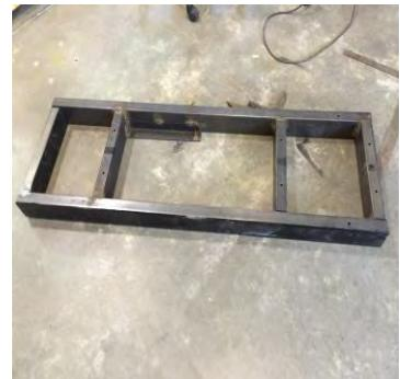
*Figure 19: The horizontal metal frame*
