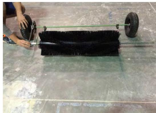
*Figure 14: Only one drive wheel is connected to the bristle system using gears and a chain mechanism*
