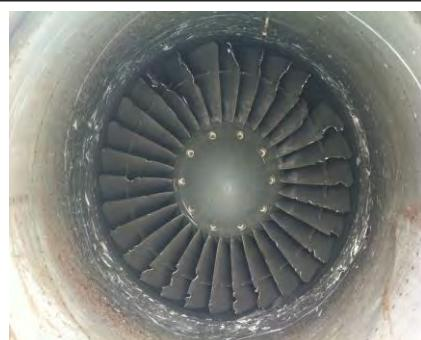
*Figure 4: Damaged fan blades cause by FOD*
