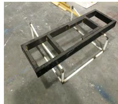
*Figure 18: The horizontal frame welded to the framework*
