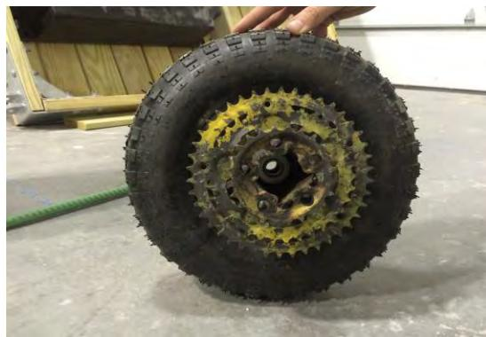
Figure 15: The gear driving drive wheel
