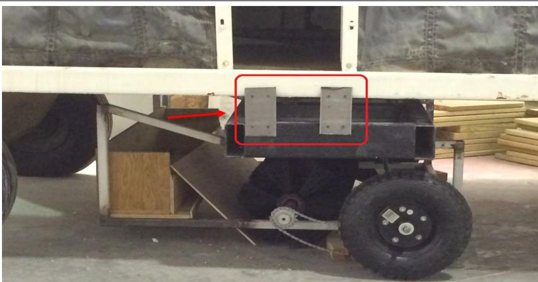
*Figure 20: The sheet metal bolted to the flange of the horizontal frame and the flange of the baggage cart*
