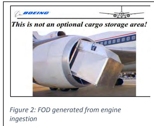
*Figure 2: FOD generated from engine ingestion*
