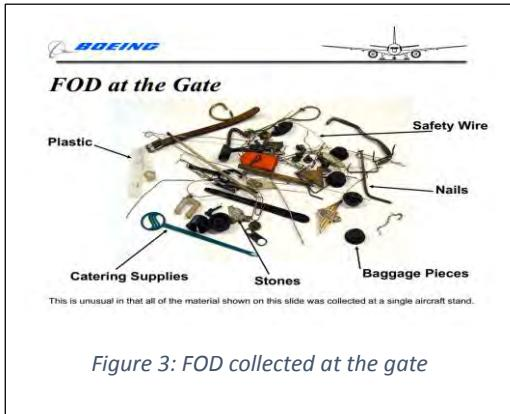
*Figure 3: FOD collected at the gate*
