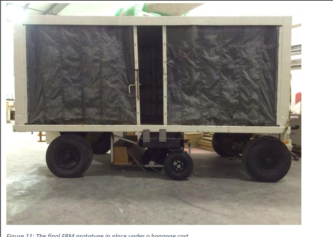
Figure 11: The final FRM prototype in place under a baggage cart
