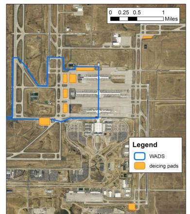
Figure 1.2. Map of the West Airfield Diversion System and deicing pads at DIA.
