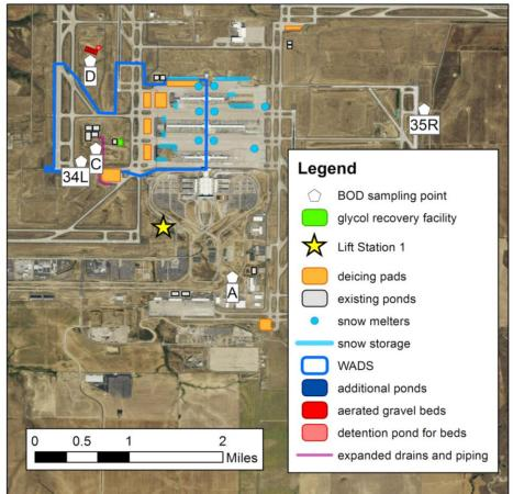
Figure 4.1. Map of deicing infrastructure at DIA and locations of proposed alternatives.
