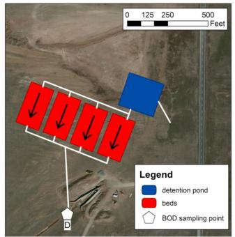
Figure 6.2. Plan view of proposed layout for subterranean aerated gravel beds and corresponding detention pond near sampling location D.
