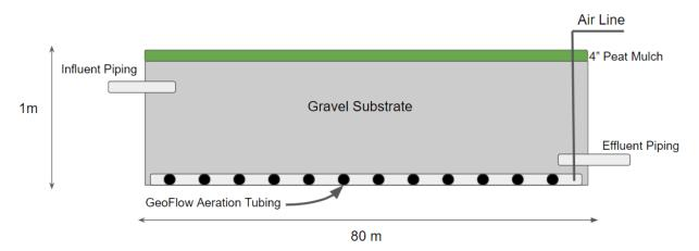
Figure 6.3. Schematic of a subterranean aerated gravel bed (adapted from Nivala et al. 2013) [22].
