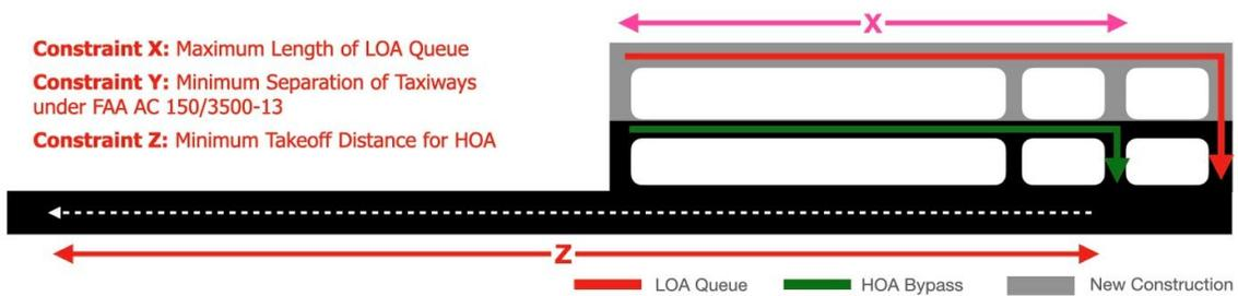
Fig. 6. Construction of a Parallel Approach Taxiway (Standard Implementation 2)
