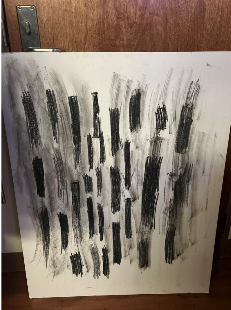
[Figure 14: Device testing surface used to imitate rubber-covered runway]
