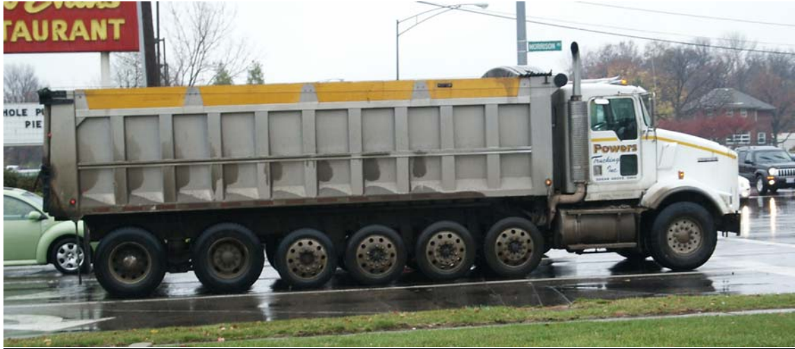
Figure 7 Multi-Axle Specialized Hauling Vehicle (Ref: NCHRP Report 575)
