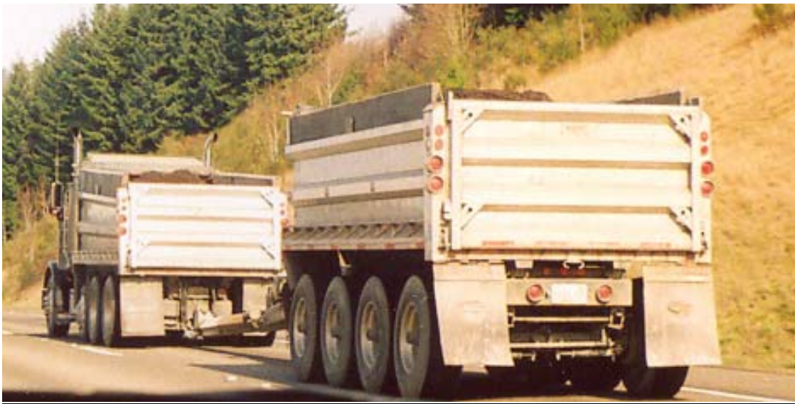
Figure 8 Truck with Tridem and Quad Axles
