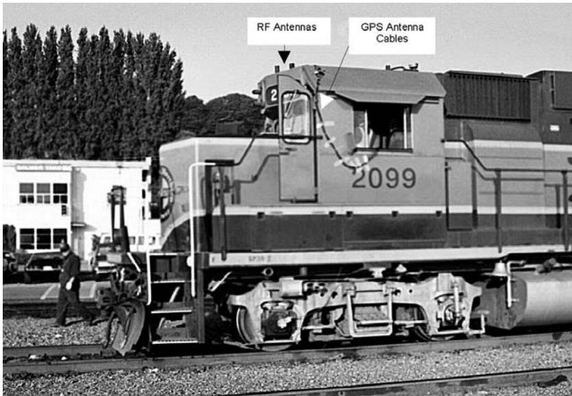
FIGURE 10. Burlington Northern Santa Fe (BNSF) GPS Work Train 2099 (Balmer Yard, Seattle, Washington, October 2000)
