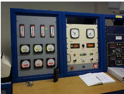
Figure 26 - Engine Control System
