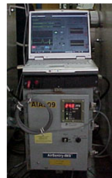
Figure 31 – IMS and Data Acquisition Computer
