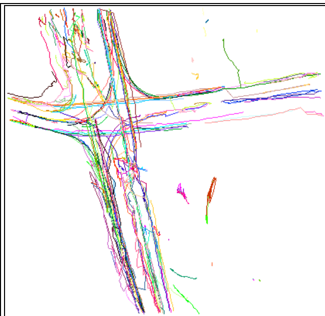
FIGURE 3b Vehicular traffic trajectories at the Hartsdale intersection, old design, camera at 35 feet
