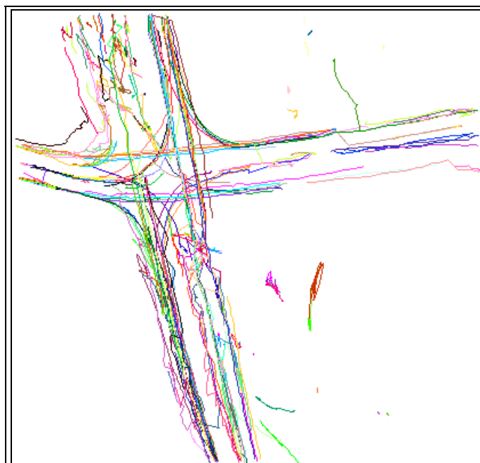
FIGURE 8b Vehicular traffic trajectories at the Hartsdale intersection, old design, camera at 35 feet
