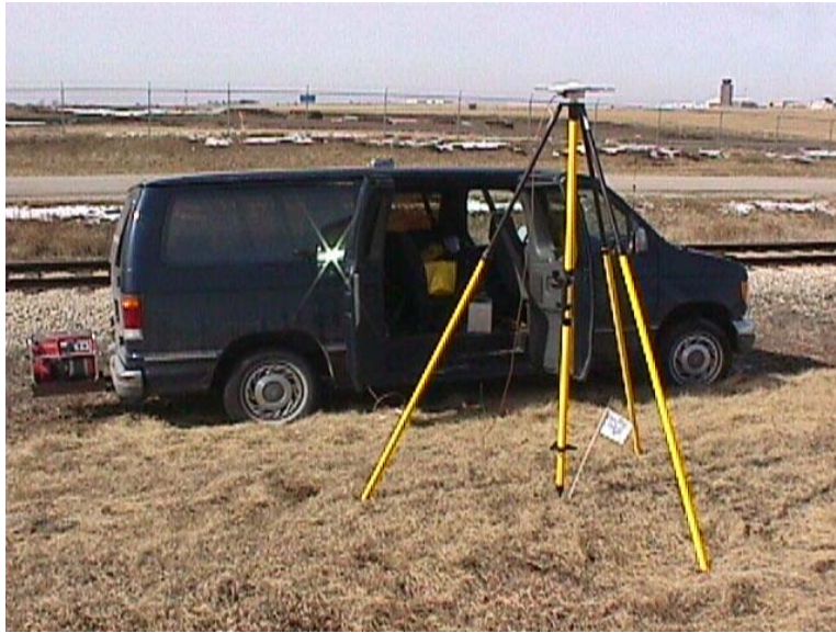
Figure 3 Van with Base Station Antenna
