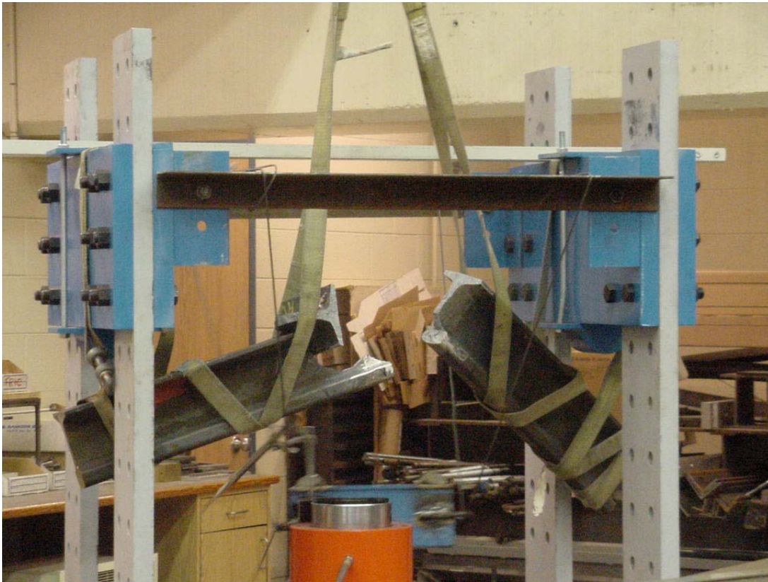
FIGURE 12. Rail weld breaking in four-point bend fixture at Portland State University.
