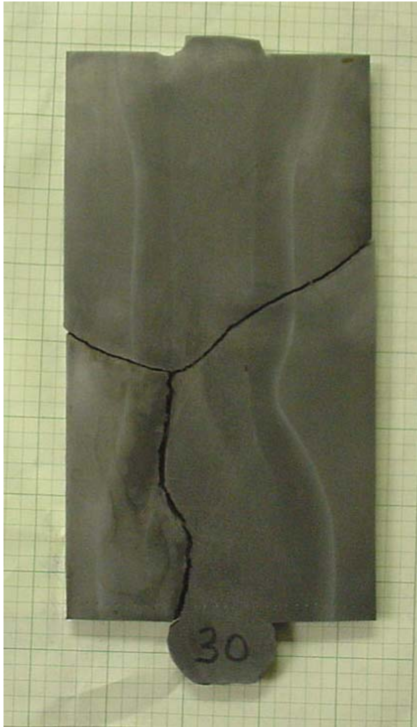
FIGURE 6. Etched macro cross-section of weld #30.
