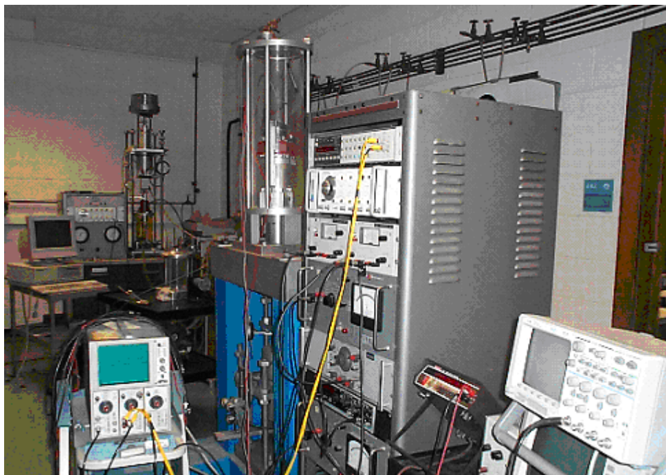
FIGURE 5 Oscilloscopes and Voltage Generators Attached to the Resonant Column Device
