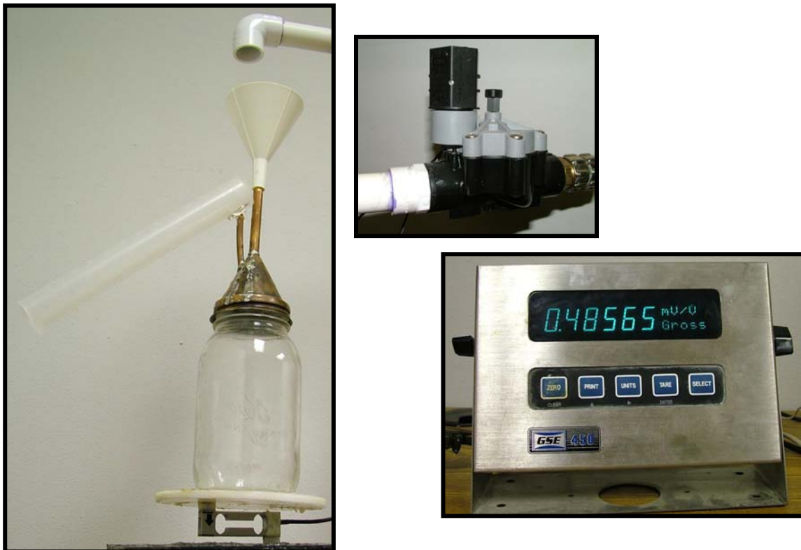
Figure 24 – Photographs of Automated Specific-Gravity Measurement System
