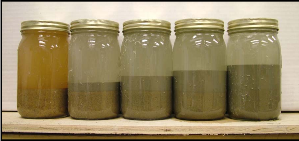
Figure 17 – Visual Demonstration of Different Cementitious-Materials-to-Sand Ratios ( CM/S )
