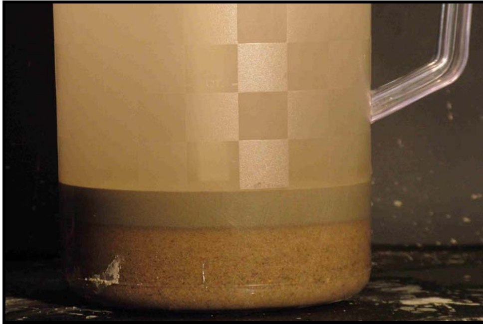
Figure 18 – Sedimentation Chamber for Measuring Cementitious-Materials-to-Sand Ratio ( CM/S )
