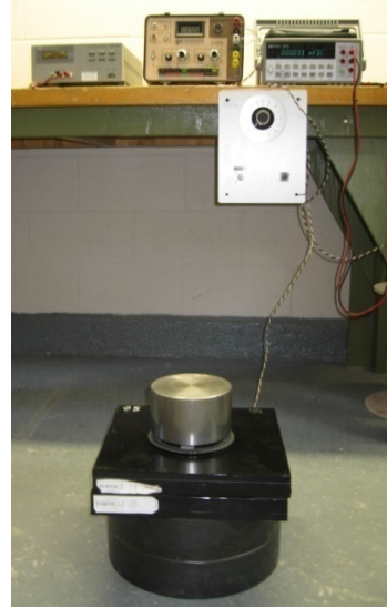
Fig. 3.7 - Calibration test of BCD plate
