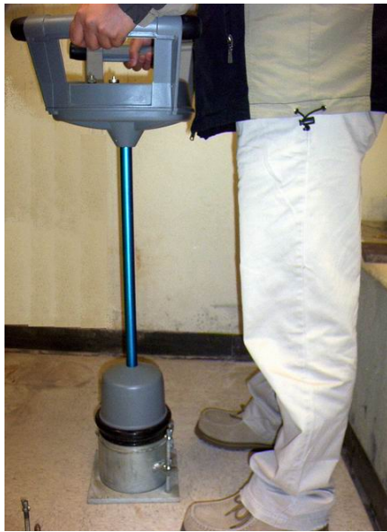
(a) BCD Test on Compaction Mold
