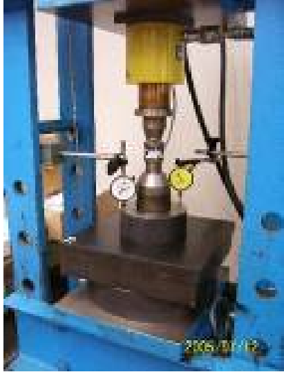
Fig. 3.6 – Obtaining the block modulus
