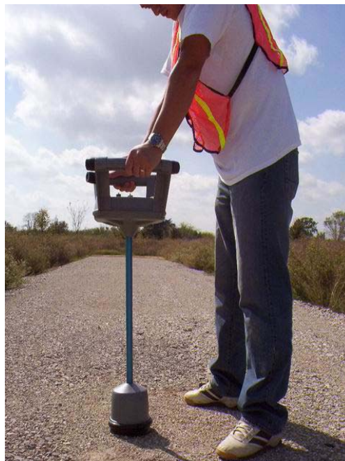
Fig. 5.5 - The BCD field test
