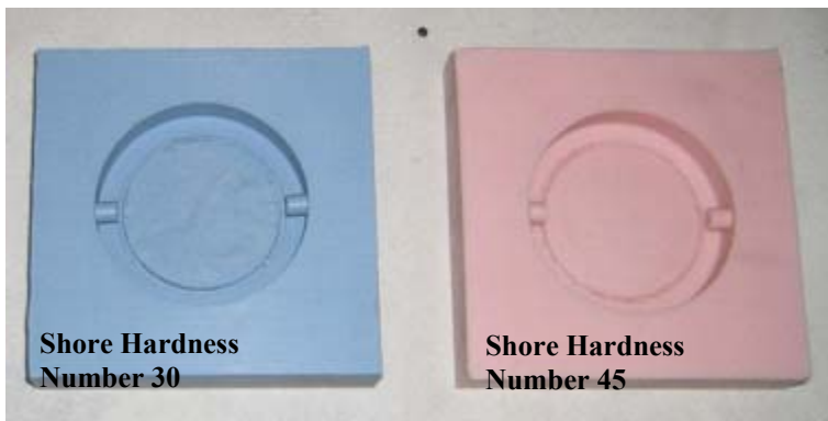
FIGURE 4.3 ABCD silicone molds flexible (left) and stiff (right). In the final version of these molds, only one of the two protrusions has been retained.
