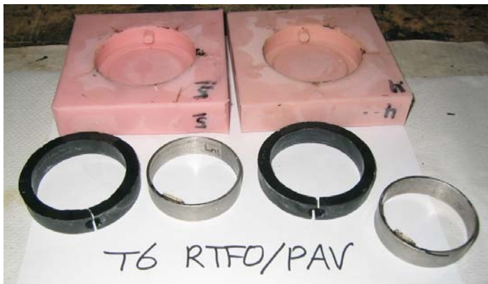
FIGURE 4.6 Cracked test specimens removed from ABCD rings and molds.
