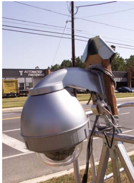
FIGURE 2. PTZ camera mounted on aerial lift platform
