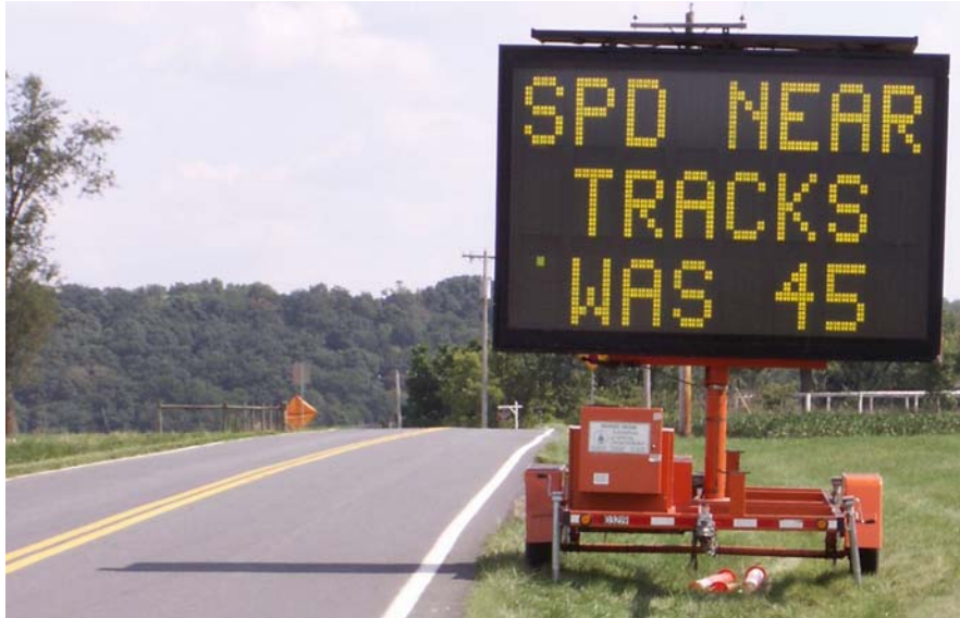
FIGURE 16. CMS downstream of grade crossing
