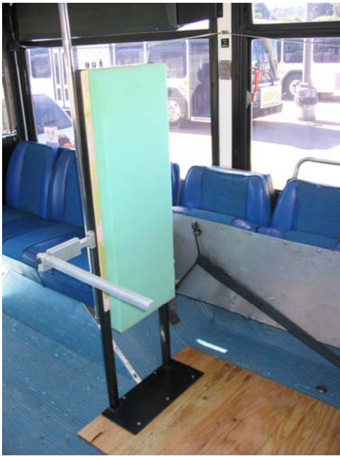
Figure 20 -A rear facing wheelchair securement station with a movable armrest. It is mounted immediately behind a wheel well in the LTD test bus.
