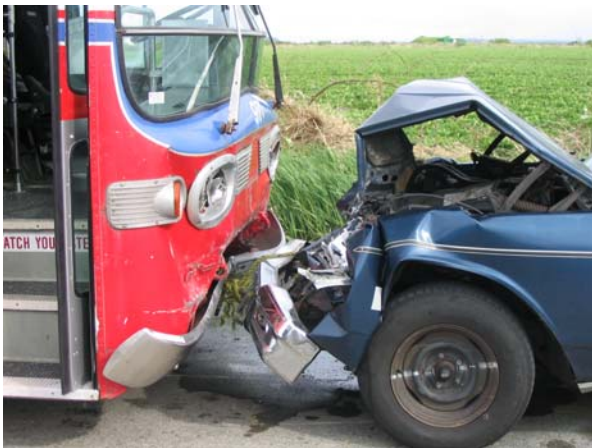
FIGURE 14 – The car and bus (rolled back into pre-crash position) showing the damage resulting from a 30mph full frontal crash. (BC Transit)
