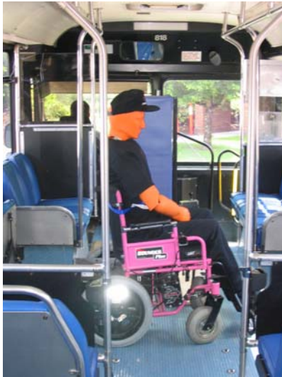
FIGURE 18 – The power wheelchair in position for side facing tests. No rear, forward, or right side constraints were used for this test of a simplest possible side facing securement station. (LTD Vehicle)
