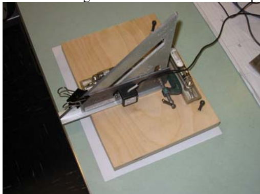
FIGURE 5 – The calibration apparatus for checking the offset voltage and calibration constant for each axis of the accelerometers.
